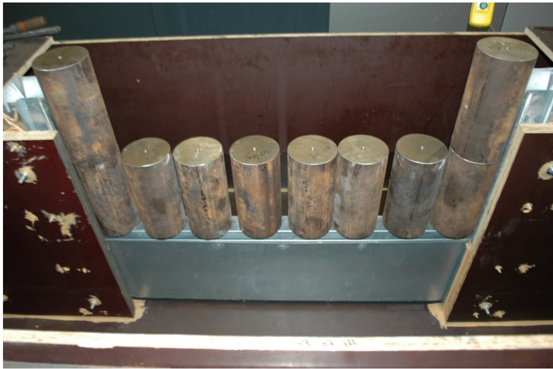
Photo C.1 View of inside of test specimen 300 mm, water at the outside
