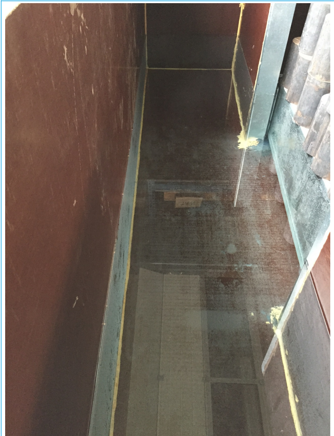
Photo C.7 View of the inside of the test specimen 500 mm, water at the inside
